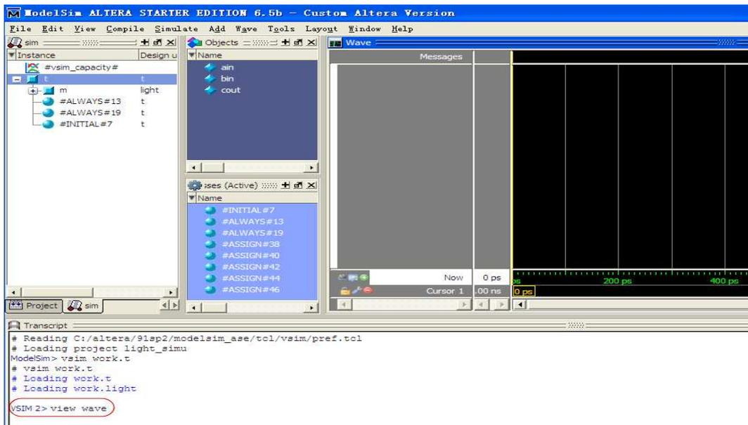
Figure 38.Using the command to open Wave Window
