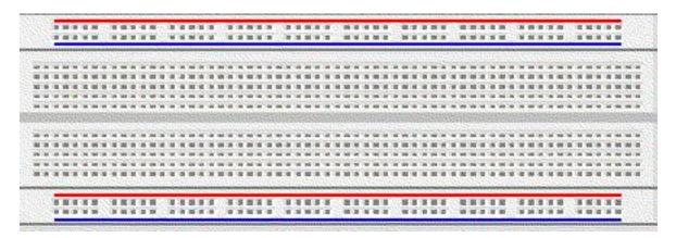
The bread board has many strips of metal (copper usually) which run underneath the board. The metal strips are laid out as shown below.
