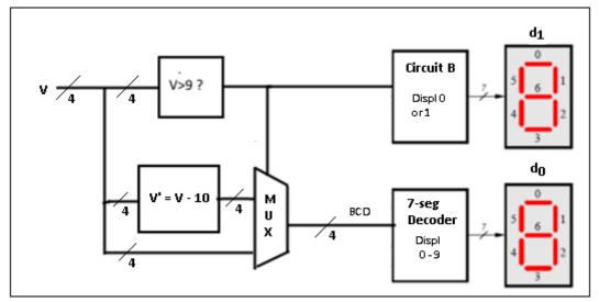
The above diagram shows a 4-bit number V converted into a 2-digit BCD. For example, if V = binary 1100 (decimal 12) then d1 displays 1 and d0 displays 2. If V = binary 0011 then d1 displays 0 and d0 displays 3. The comparator labeled "V > 9?" outputs 1 if true, 0 if false. That result gets displayed on 7-segment display d1, and makes the MUX select V or V-10 to display on d0.
