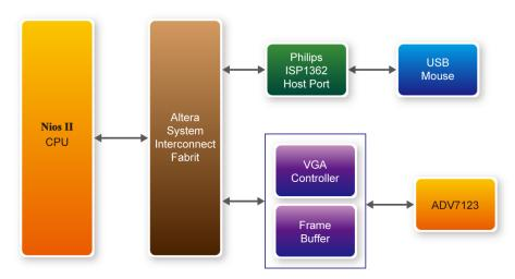
Figure 6-3 Block diagram of the USB paintbrush demonstration
