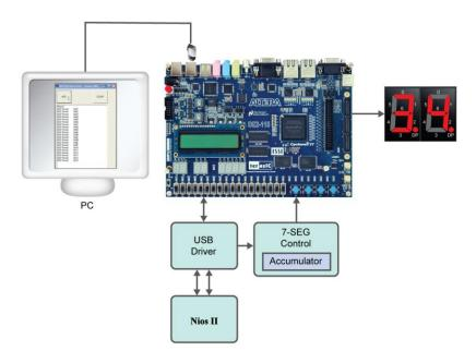
Figure 6-6 Setup for the USB device demonstration
