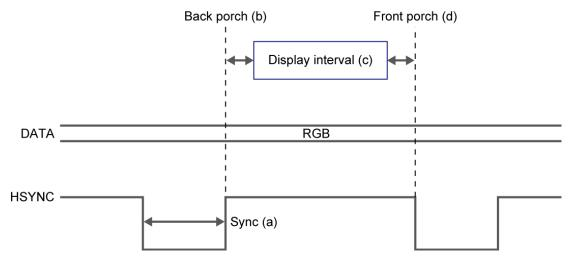
Figure 4-22 VGA horizontal timing specification
