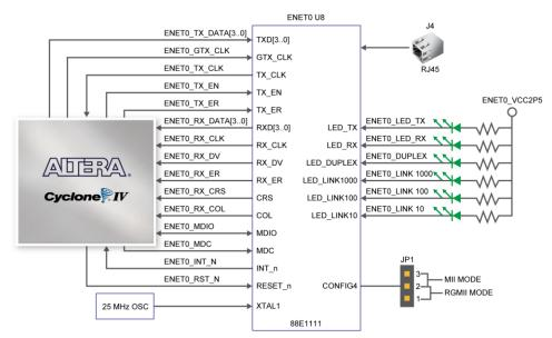
Figure 4-27 **Connections between FPGA and Ethernet**
