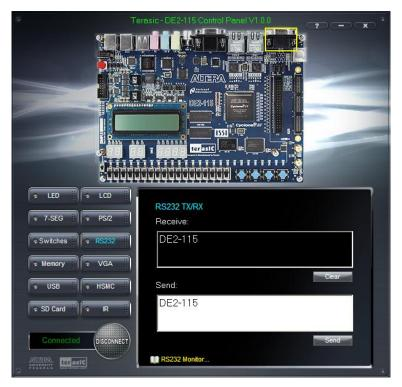
Figure 3-11 RS-232 Serial Communication
