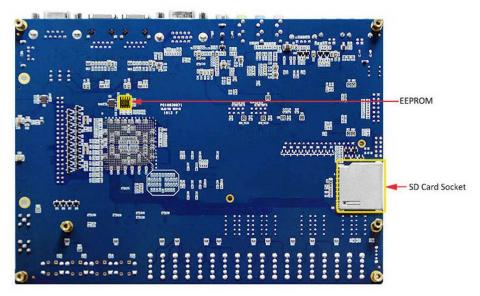
Figure 2-2 The DE2-115 board (bottom view)
