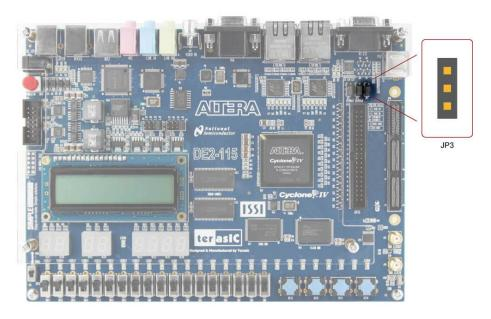
Figure 4-2 The JTAG chain configuration header
