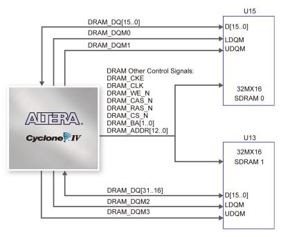
Figure 4-34 Connections between FPGA and SDRAM
