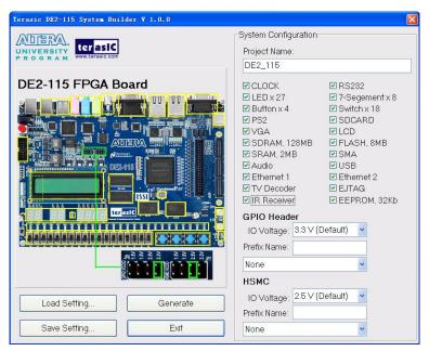
Figure 5-2 The DE2-115 System Builder window
