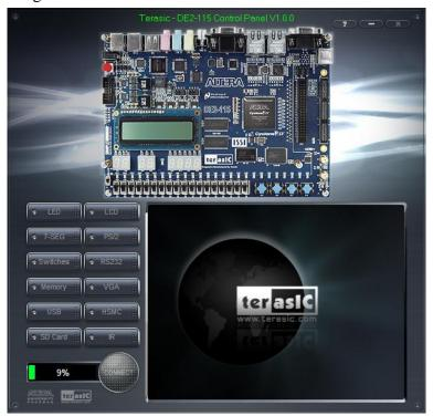
Figure 3-1 The DE2-115 Control Panel
