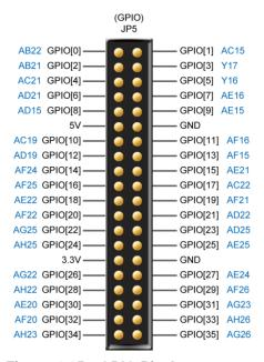
Figure 4-15 GPIO Pin Arrangement
