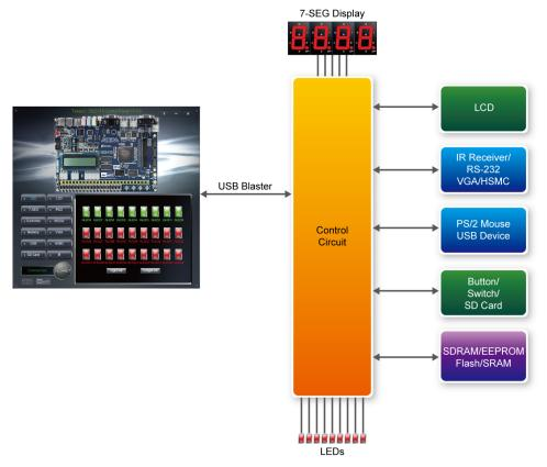
Figure 3-2 The DE2-115 Control Panel concept
