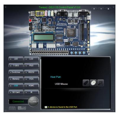
Figure 3-8 USB Mouse Monitoring Tool
