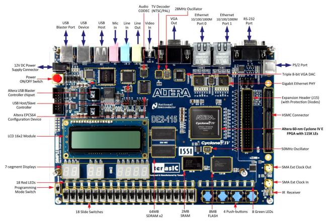
Figure 2-1 The DE2-115 board (top view)
