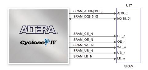
Figure 4-33 Connections between FPGA and SRAM
