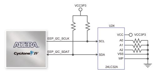
Figure 4-36 Connections between FPGA and EEPROM
