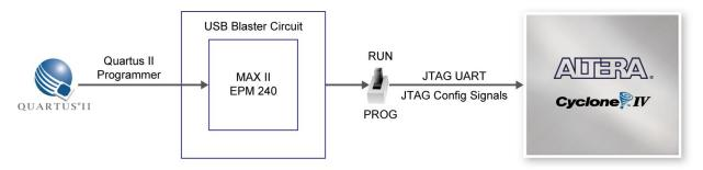
Figure 4-3 The JTAG configuration scheme
