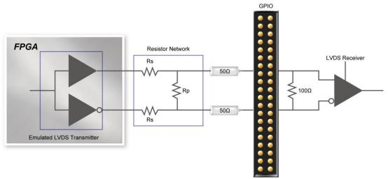
Figure 4-19 Using Emulated LVDS on GPIO
