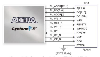
Figure 4-35 Connections between FPGA and Flash
