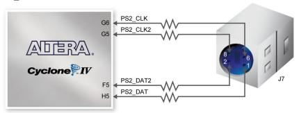
Figure 4-25 Connection between FPGA and PS/2
