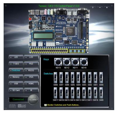
Figure 3-6 Monitoring switches and buttons
