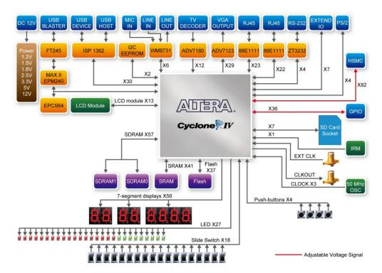
Figure 2-3 Block Diagram of DE2-115
