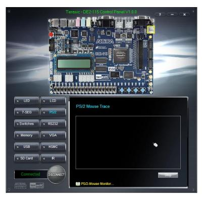
Figure 3-9 PS/2 Mouse Monitoring Tool
