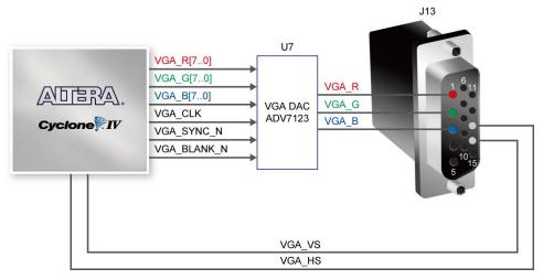
Figure 4-21 Connections between FPGA and VGA
