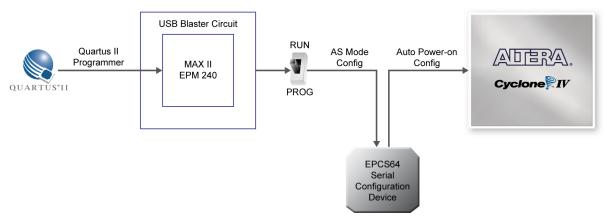
Figure 4-5 The AS configuration scheme
