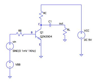
Consider the amplifying circuit provided in figure. Select adequate values for RB, RC and VBB so that the DC bias point is set at VCE=4.5V and IC=10 mA.
