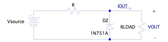
NOTE: Use the programmable voltage supplies VP+ and VP- to generate the required Vsource
