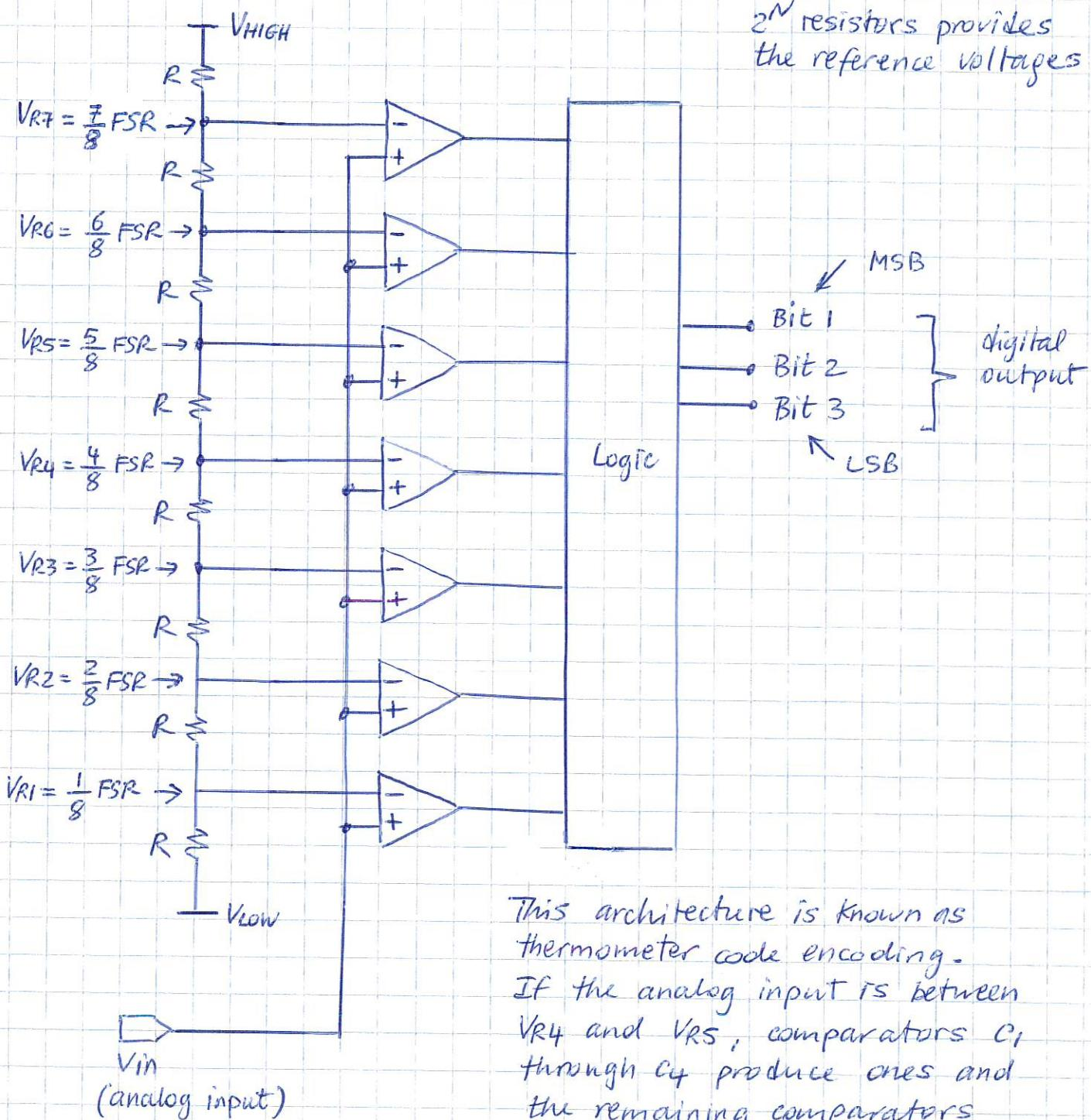
This architecture is known as thermometer code encoding. If the analog input is between  $V_{R4}$  and  $V_{R5}$ , comparators  $C_1$  through  $C_4$  produce ones and the remaining comparators produce zeros.
