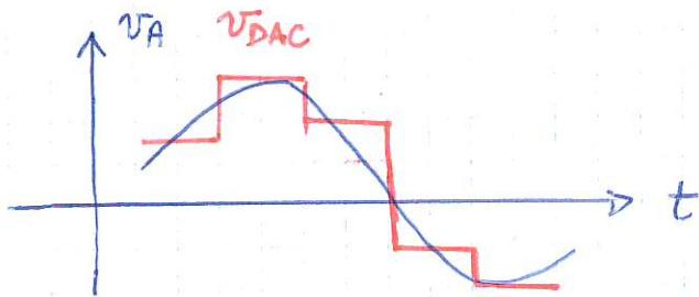
the staircase waveform at the output of a DAC can be filtered to obtain a smoother waveform ( $\rightarrow$  through a LPF).  $\Rightarrow$  the filter will introduce a time delay.
