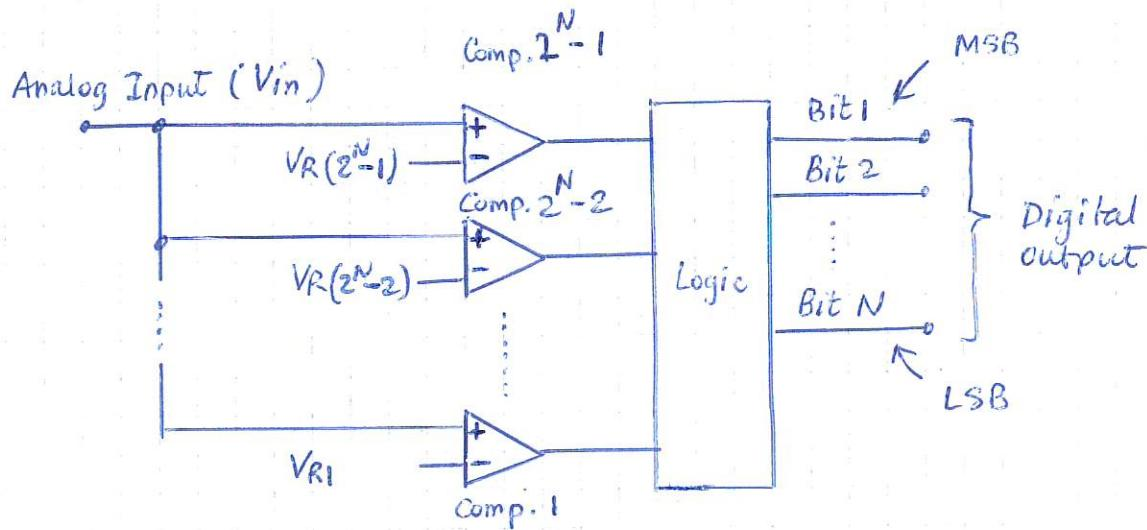
The outputs of the comparators are processed by an encoder block to provide the  $N$  bits of the output digital word.
