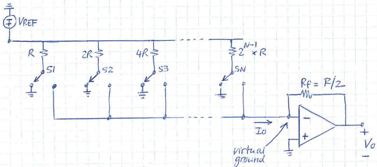
The switches are controlled by an  $N$ -bit digital input  $b_1, b_2 \dots b_N$ . The total current  $I_O$  that will flow through the feedback resistor of the op-amp is proportional to the digital word.
