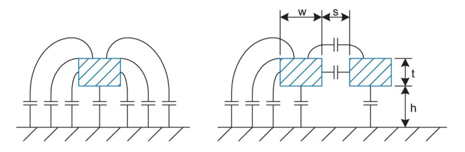
FIG 4.34 Effect of fringing fields on capacitance
