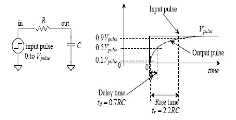
Figure 2.21 Rise and delay times in an RC circuit.
