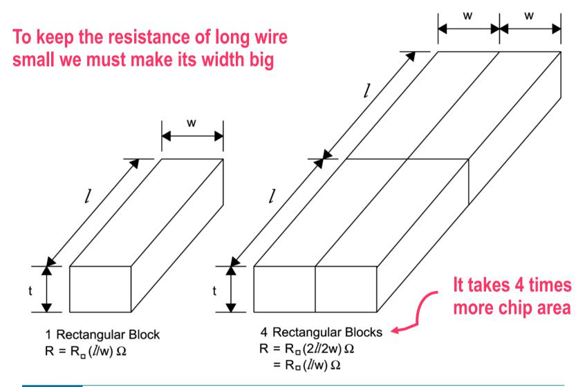
FIG 4.32 Two conductors with equal resistance
