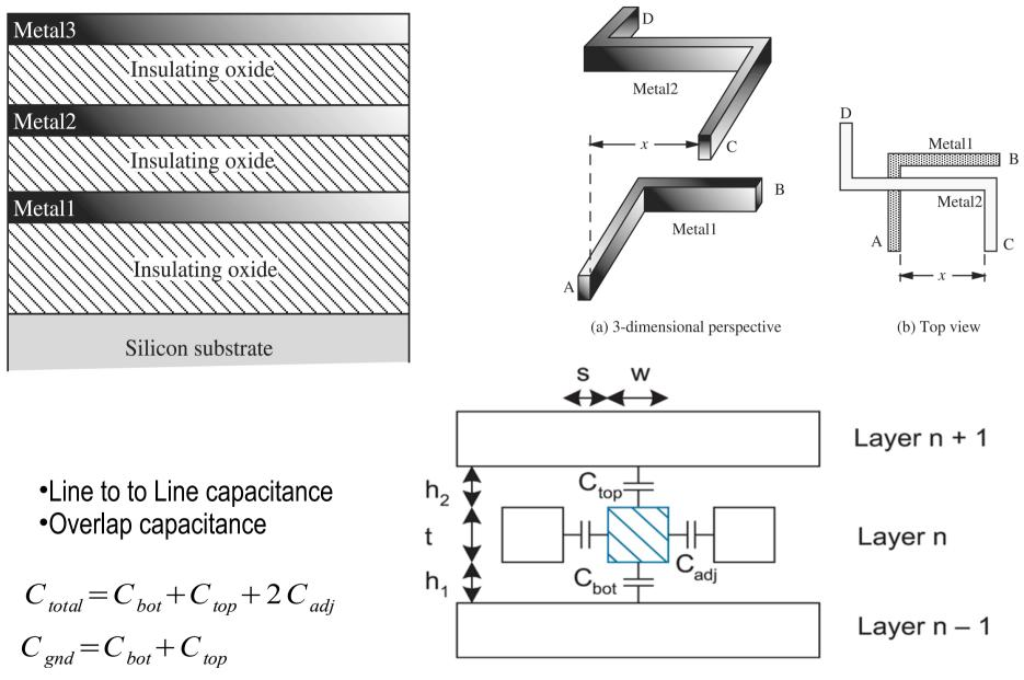
FIG 4.36 Multilayer capacitance model
