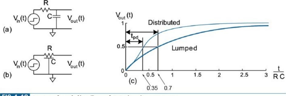
FIG 4.48 Lumped and distributed RC circuit response
