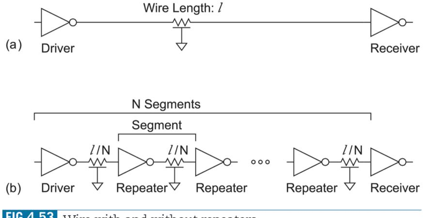
**FIG 4.53** Wire with and without repeaters
