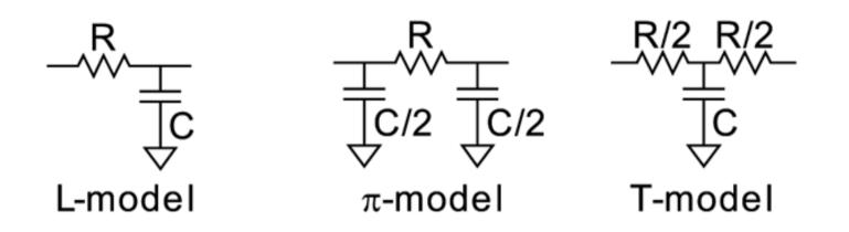
**FIG 4.38** Lumped approximation to distributed RC circuit
