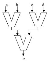
Recommendation: use parenthesis to control the structure of the synthesized logic.
