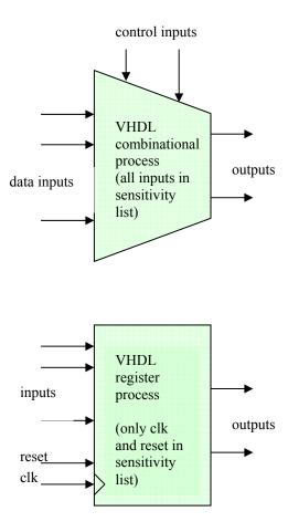
Note that the register processes may include some combinational logic, but all effects of that logic must end up in the D-input of a register instantiated in the process. The inputs should not feed non-registered output logic. If it did, the output logic wouldn't simulate correctly, since its inputs are not in the process's sensitivity list.
