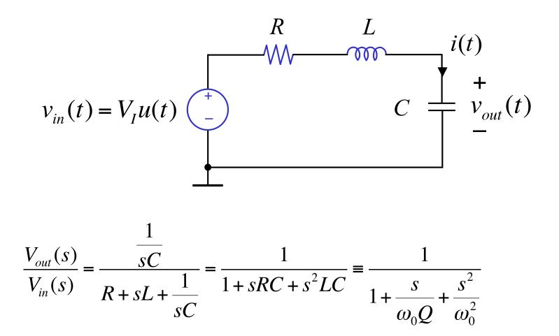
$$\omega_0^2 = \frac{1}{LC}; \quad Q = \frac{1}{\omega_0 RC} = \frac{\sqrt{L/C}}{R} \equiv \frac{Z_0}{R}$$
