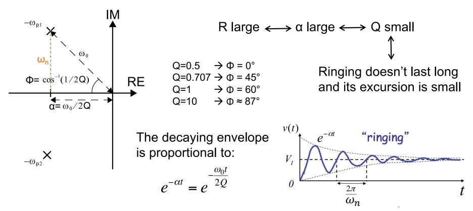
Rule of thumb: Q is roughly equal to the number of cycles of ringing.
