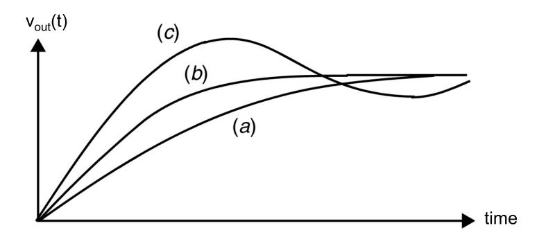
(a) Overdamped Q < 0.5  $(\alpha > \omega_0 \Leftrightarrow \zeta \equiv \alpha / \omega_0 > 1)$
