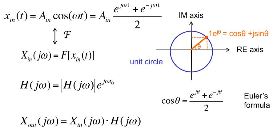
$$X_{out}(j\omega) = X_{in}(j\omega) \cdot H(j\omega) = X_{in}(j\omega) \cdot |H(j\omega)| \cdot e^{j\omega t_0}$$
