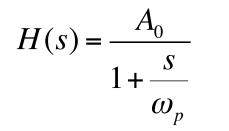
First order low pass transfer function. This is the most commonly encountered transfer function in electronic circuits
