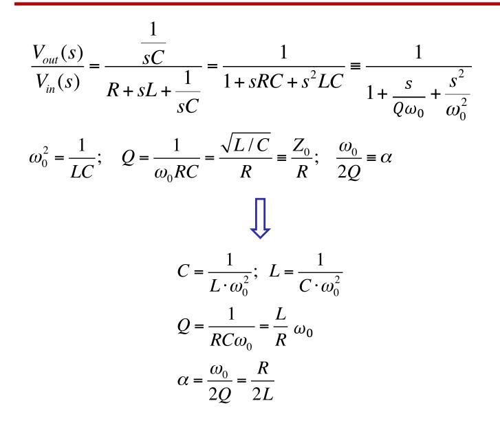
$$s^{2} + s \cdot \frac{\omega_{0}}{Q} + \omega_{0}^{2} = 0 \Leftrightarrow s^{2} + s \cdot 2\alpha + \omega_{0}^{2} = 0 \Leftrightarrow s_{1,2} = -\alpha \mp \sqrt{\alpha^{2} - \omega_{0}^{2}}$$
