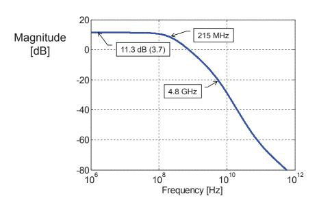
Calculated values: |A<sub>v0</sub>|=12 dB (4.0), f<sub>p1</sub> = 200 MHz, f<sub>p2</sub>= 5.8 GHz
