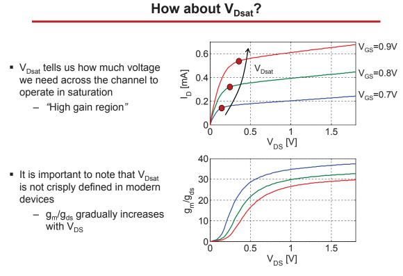
It turns out that 2/(g<sub>m</sub>/l<sub>D</sub>) is a reasonable first-order estimate for V<sub>Dsat</sub>
