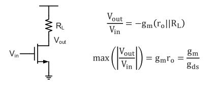
Square law:  $g_m r_o = \frac{1}{\lambda} \frac{g_m}{I_D} = \frac{1}{\lambda} \frac{2}{V_{OV}}$  A very poor model
