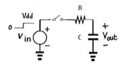
Given an RC circuit which input is a voltage step from 0 to  $V_{\rm DD}$ , and which output is the voltage on the capacitor, derive the circuit delay time (time it takes the output voltage to reach the 50% of its final value), and the circuit rise time (time it takes the output voltage to go from the 10% to the 90% of its final value).
