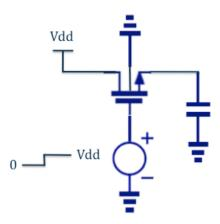
Given the simple nMOS pass transistor circuit shown compute the max voltage that is possible to pass to the load capacitor (CL=16fF). Design the nMOS pass transistor to be unit size in TSMC 180nm technology.
