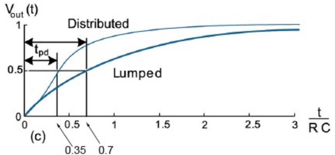
**FIG 4.48** Lumped and distributed RC circuit response
