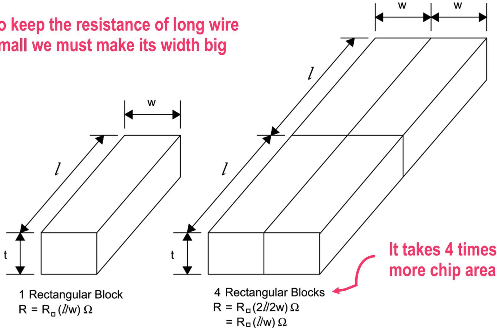
**FIG 4.32** Two conductors with equal resistance
