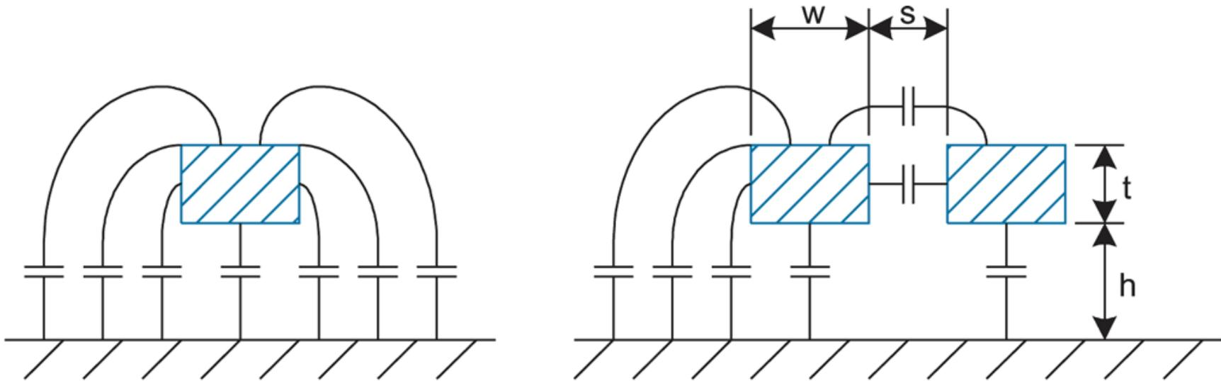
**FIG 4.34** Effect of fringing fields on capacitance
