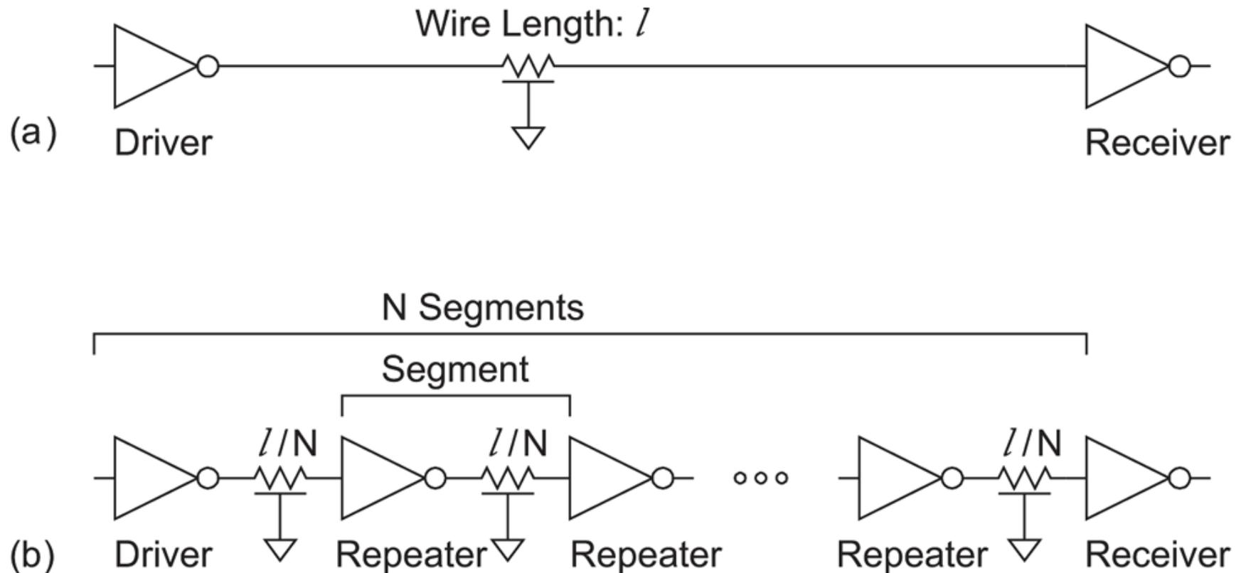
**FIG 4.53** Wire with and without repeaters
