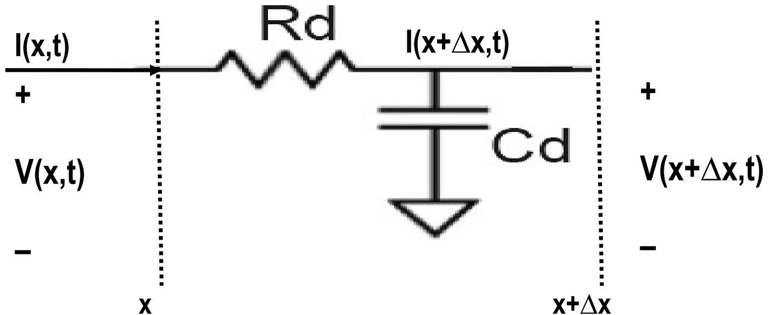
$$\begin{cases} V(x,t) - V(x+\Delta x,t) = R_d I(x,t) \\ I(x,t) - I(x+\Delta x,t) = C_d \frac{\partial V(x+\Delta x,t)}{\partial t} \end{cases}$$
