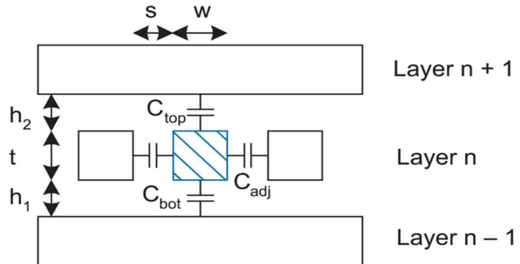
**FIG 4.36** Multilayer capacitance model
