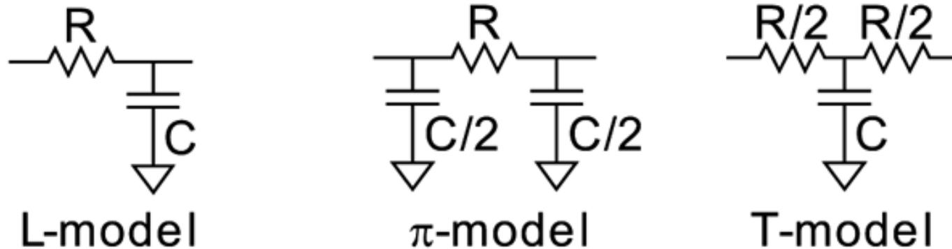
**FIG 4.38** Lumped approximation to distributed RC circuit
